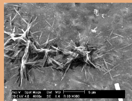
Figure 2. Fritted glass produced with 30 mass% WDR
