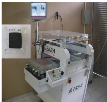
Figure 1. Sieve-printing apparatus for Membrane-Electrode-Assembly (MEA) production
