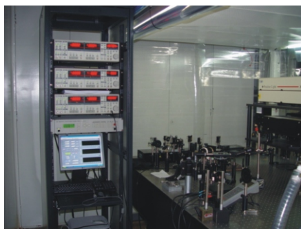
Figure 11. Setup for studying ultrafast dynamic process with the pump and probe technique under development in Center of Lasers of IPEN
