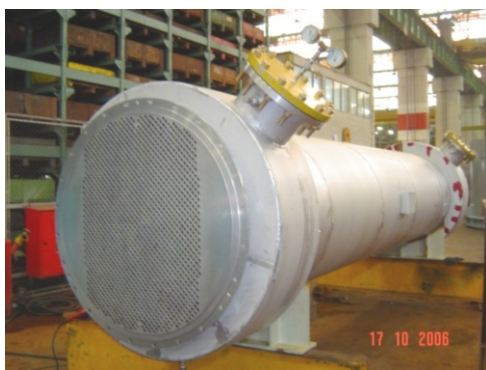
Figure 12. New heat exchanger
