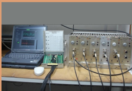
Figure 9. Isolating amplifiers used to data pre-processing in the noise analysis methodology
